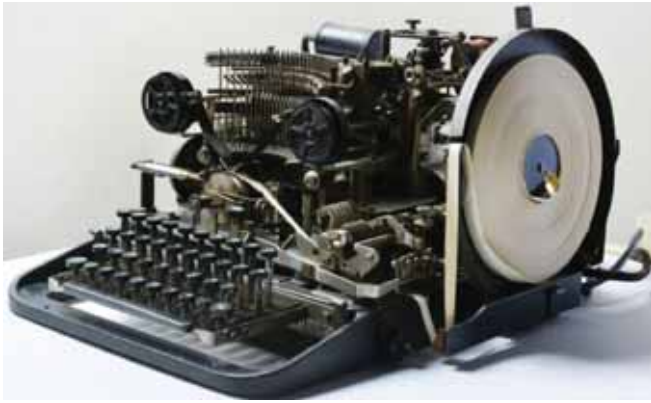
The teleprinter for the Lorenz cipher machine, which Hitler used to message his top generals
